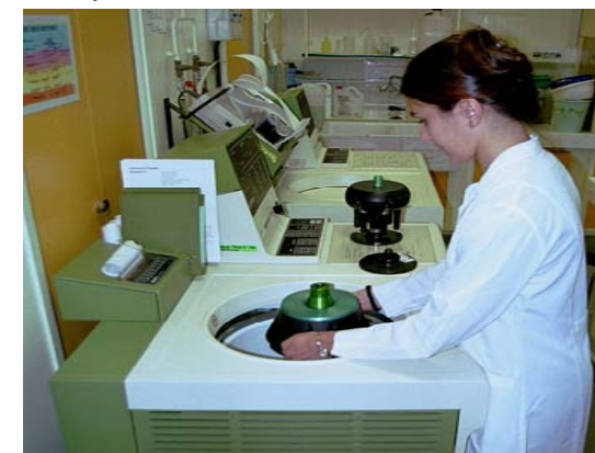
Ultracentrifuges equipped with swinging-bucket and fixed angle rotors
