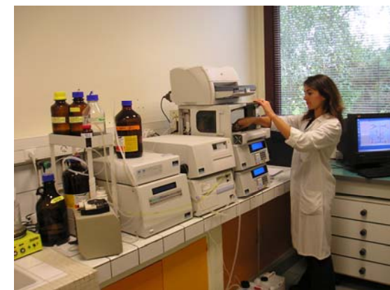
High-Performance Liquid Chromatograph coupled with a fluorimeter (HPLC-Fluo)
