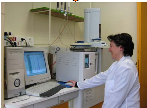
Gas-liquid chromatograph-FID equipped with a H 2 generator (GC-FID)
